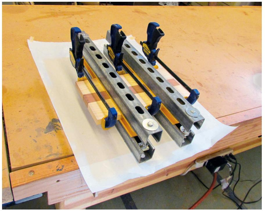
Here's a surefire method to ensure flat glue-ups. Use cauls, top and bottom, made from <u>Unistrut</u>. This steel channel is used for light-duty structural support in electrical and plumbing work. Sometimes called Superstrut, it's available in the electrical department of many home centers in 10' lengths.
